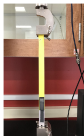
Figure 1. Peeling Off results of NMC electrodes with 5% PAN and 7.5% PVDF as binders, with a photo of the peeling-off test setup.
