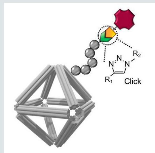
(Above) A schematic showing how “alkyne” reactive groups incorporated into peptoid sequences coating the DNA origami can conjugate with fluorophore-labeled nanocargo (such as trastuzumab) that have been modified with “azide” chemical groups (red shape). Through alkyne-azide click-chemistry reactions, the surface of peptoid-coated DNA origami can be functionalized.
