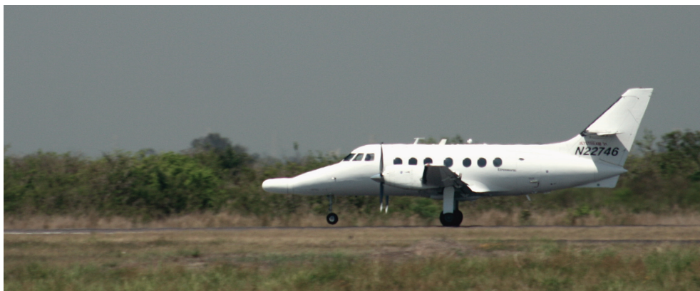
Lift-off of the Jetstream-31 aircraft during a research flight in Veracruz, Mexico. The Research Scanning Polarimeter is located in the tail of the aircraft.
