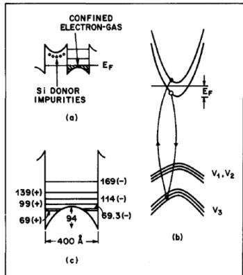
FIG. 1: (a) Model of the conduction band edge of modulation doped heterojunction superlattices.
