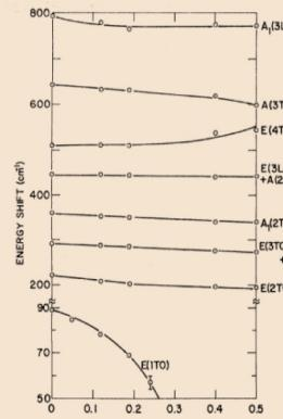
FIG. 3. Experimental results at 23°C in the tetragonal phase of the  $\text{PbTi}_{1-x}\text{Zr}_x\text{O}_3$  system. For  $x > 0.25$ ,  $E(1\text{TO})$  could not be measured because of low energy shifts and laser scattering background.
