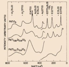
FIG. 2. Experimental Raman powder patterns measured at 23°C for three samples in the  $\text{PbTi}_{1-x}\text{Zr}_x\text{O}_3$  system. The arrows refer to the results in single-crystal  $\text{PbTiO}_3$  (Ref. 7). (Note the gain change and overlap at  $\approx 350 \text{ cm}^{-1}$ .)
