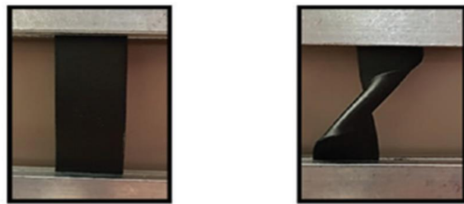
Figure 1. LbL deposition-synthesized thin film undergoing tensile stress. Source: Cho, et al. [1]
