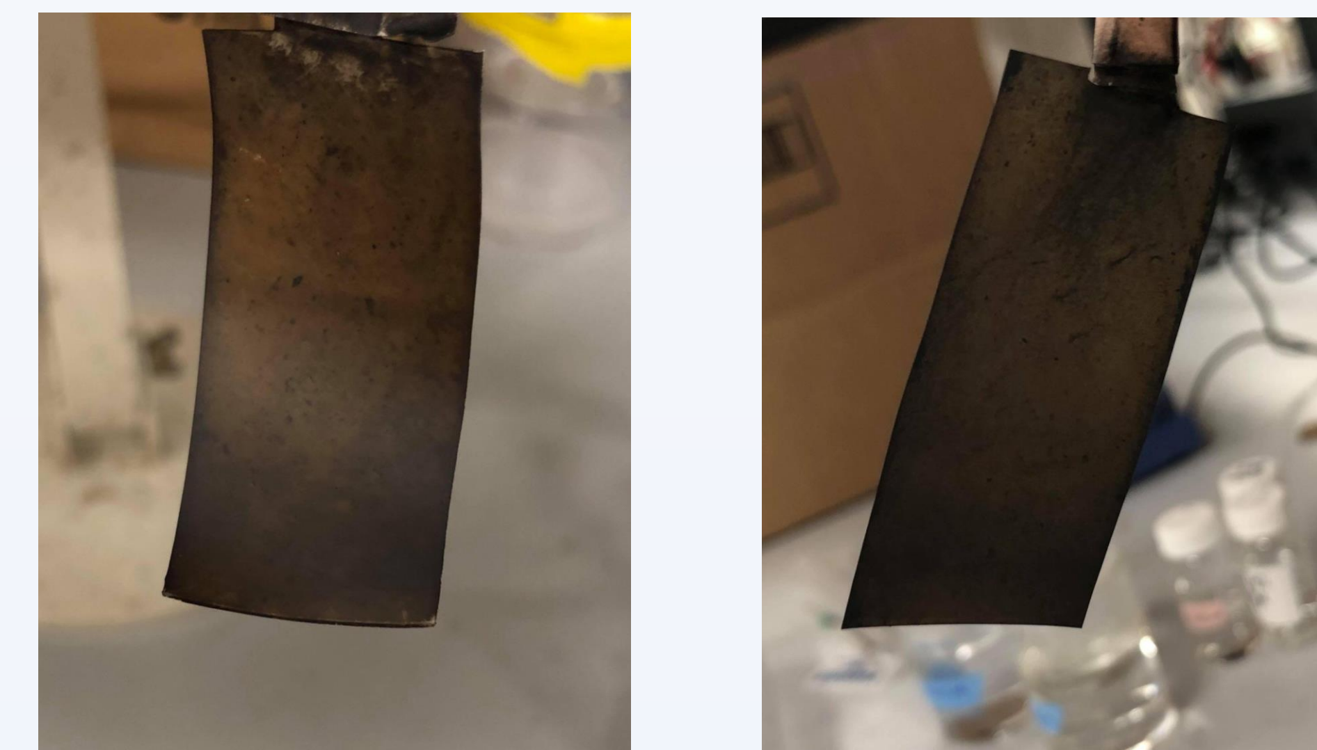
Figure 3. On left: trilayer film on PU substrate. Right: trilayer film on PET substrate.
