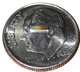
(Above) Photonic integrated chip capable of encoding data on 32 independent frequency channels on a U.S. dime for scale. Credit: Lightwave Research Laboratory / Columbia Engineering (Below) Michal Lipson & Alex Gaeta
