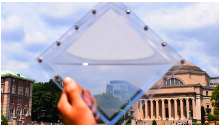
Above: The porous polymer coatings, which switch from white to transparent when wetted, can be put into plastic enclosures to make panels that control light and temperatures of buildings.
